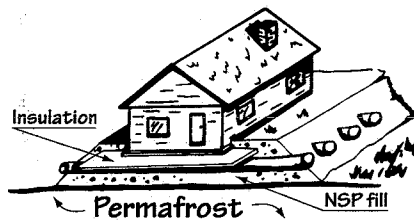
Figure 5b. Air ducts used to stabilize permafrost.
